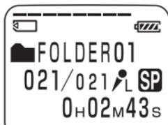
A message is being recorded as the 21st message of all 21 messages in the folder 01 in SP mode with L (low) microphone sensitivity.
