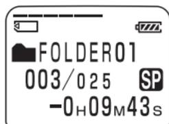
In the stop and recording mode: The remaining recording time indication.
