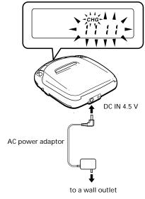
**4** When fully charged, "CHG" disappears. Disconnect the AC power adapto
