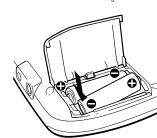
When to replace the dry batteries When the battery becomes weak, i indication flashes in the display. If the "Lo ba tt" appears in the display, replace all the batteries with new ones, because the batteries are used up.
