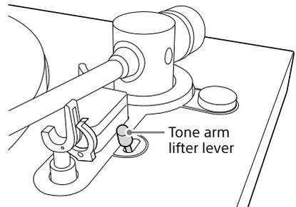
To stop the playback before it finishes, push the tone arm lifter lever toward the back of the turntable.
