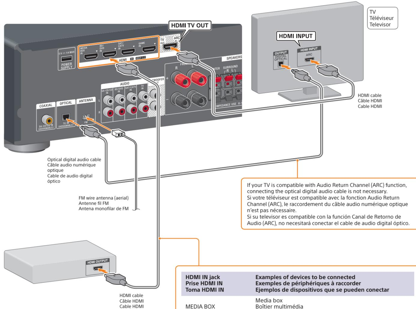
If your TV is compatible with Audio Return Channel (ARC) function, connecting the optical digital audio cable is not necessary.
