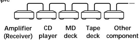
In the CONTROL A1II control system, the control signals flow both ways, so there is no distinction of IN and OUT jacks. If a component has more than one CONTROL A1II jack, you can use either one, or connect different components to each jack.
