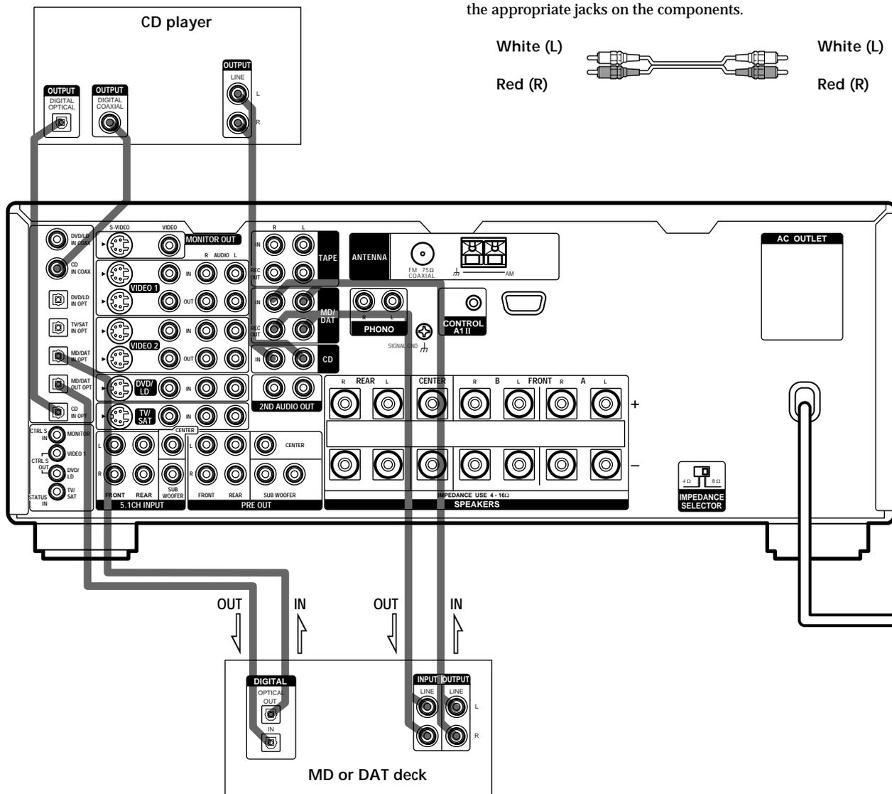
\* Make either coaxial or optical connections. We recommended making coaxial connections instead of optical connections.
