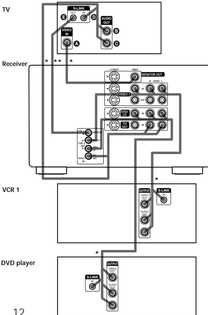
\* Audio/video/control S connecting cord (Pull the video cord away from the supplied audio/video/control S cable for connection **A**.)
